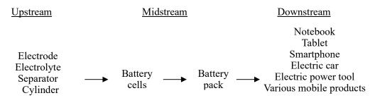
For the upstream raw material, a battery cell is mainly formed by rour components, namely electrodes (cathode and anode), electrolyte, separator and cylinder. However, the requirements for functions and materials may differ according to the battery types.
